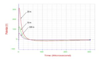
Fig. 5: Computed GPR values at various distaces from configuration 5, installed at site 1 injected at 16 kA.
