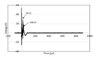
Fig. 2: Measured voltage traces at various distances from a single rod electrode, installed at site 1, injected at 100 kV.
