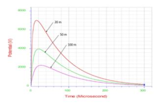
Fig. 4: Computed GPR values at various distances from configuration 5, installed at site 1 injected at 4 kA.
