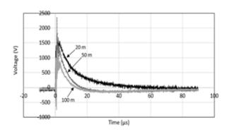
Fig. 3: Measured voltage traces at various distances from a single rod electrode, installed at site 2, injected at 100 kV.
